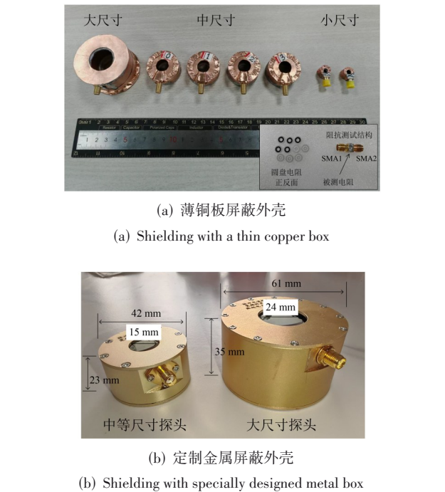
图 4 设计制作的三种尺寸的电流探头 Figure 4 Three different sizes of designed current probes
